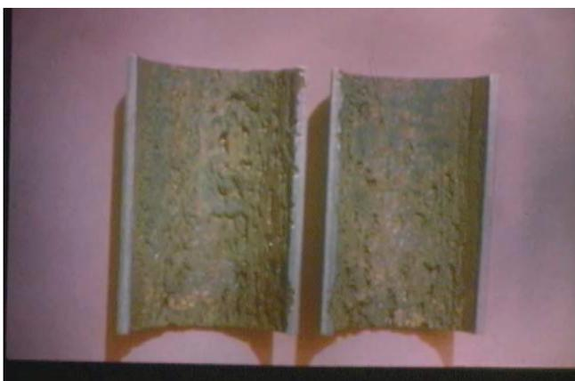
Figure 2. Pipeline corrosion pitting.
